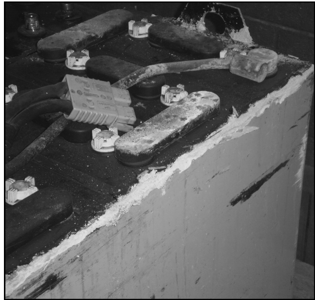
Tray corrosion can shorten battery life significantly. It is most often caused by overwatering.
