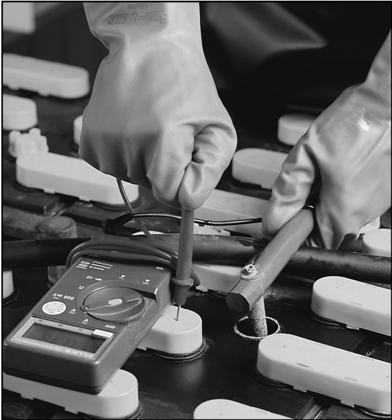
If any doubt exists as to whether a cell should be removed from the battery for inspection or repair, the cadmium electrode test can help you make the decision.
