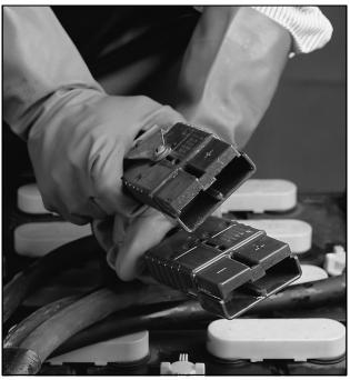
Keyed connectors eliminate the possibility of hooking up a battery to the wrong charger or vehicle. The differently keyed connector housings prevent these connectors from being interconnected.
