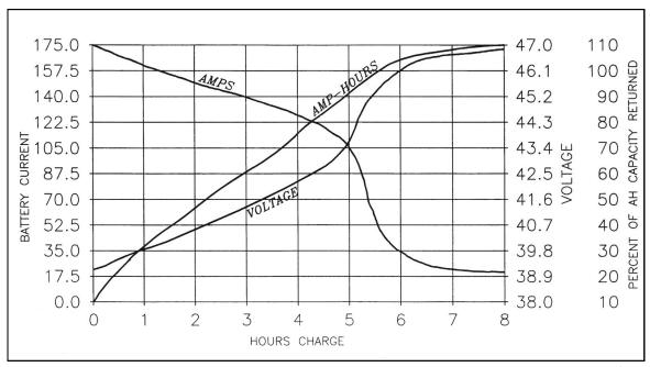
Typical Recharging Characteristics. Typical charge return to an 18-cell battery discharged at 80%, using a HAWKER<sup>®</sup> LIFEGUARD<sup>®</sup> charger.
