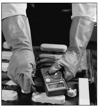
To read the individual cell voltages of a battery, place the positive lead of the voltmeter on the positive terminal of a cell, and the negative lead of the voltmeter to the negative terminal of the same cell. Cell voltages must be read to the 1/100<sup>th</sup> of a volt. [Example: 2.12, 2.09, etc.]
