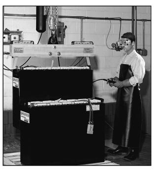
The safe way to lift a battery is to use an insulated lifting beam with safety latch. This reduces the possibility of damaging the tray and shorting the cell connectors.
