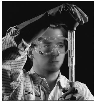
When reading a hydrometer, it is important to hold the syringe at eye level and in a vertical position. Be sure the float does not stick to the hydrometer barrel and is floating freely, not in contact with either the top or bottom of the barrel. The correct hydrometer reading is an imaginary line drawn across the scale at the lowest level of the electrolyte.
